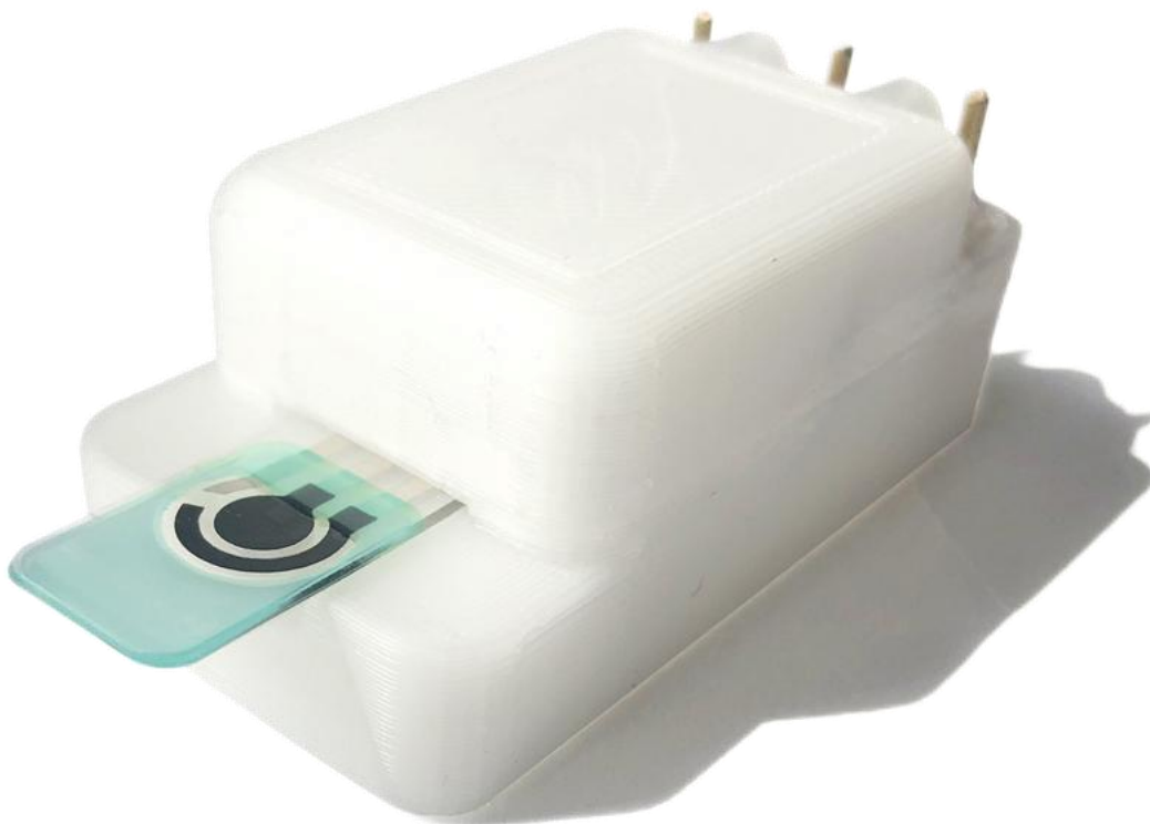
Fig.4. Electrochemical Workstation Compatible Connectors for Screen Printed Electrodes
