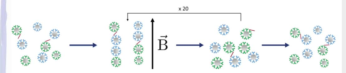
The magnetic actuation will be repeated twenty times. In between the pulses, the beads will re-orientate in order to get another chance to form a cluster.
