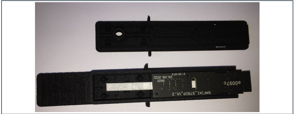
Figure 36: Assembly of the PCBA Sensor with the LFT strip in the cartridge
