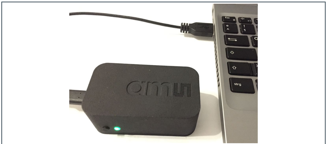
Figure 17: Green LED on the LFT Reader blinks when connected via USB to the GUI
