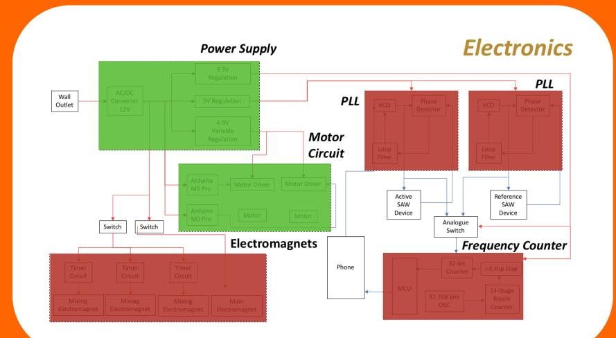
The electric circuit creates a loop searching for the resonant frequency of the device. A frequency and phase change is produced when the weight is changed by the NT-proBNP biding. Slide in case and connect the PUMP to reservoirs
