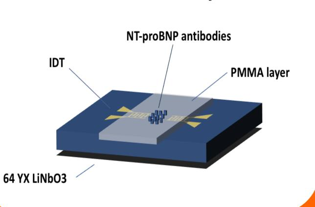
We use magnetic microparticles In order to improve the limit of detection of the sensor from a few hundred ng/ml down to a few pg/ml. [2] Use change in weight on the delay line to obtain signal Magnetic Microparticles
