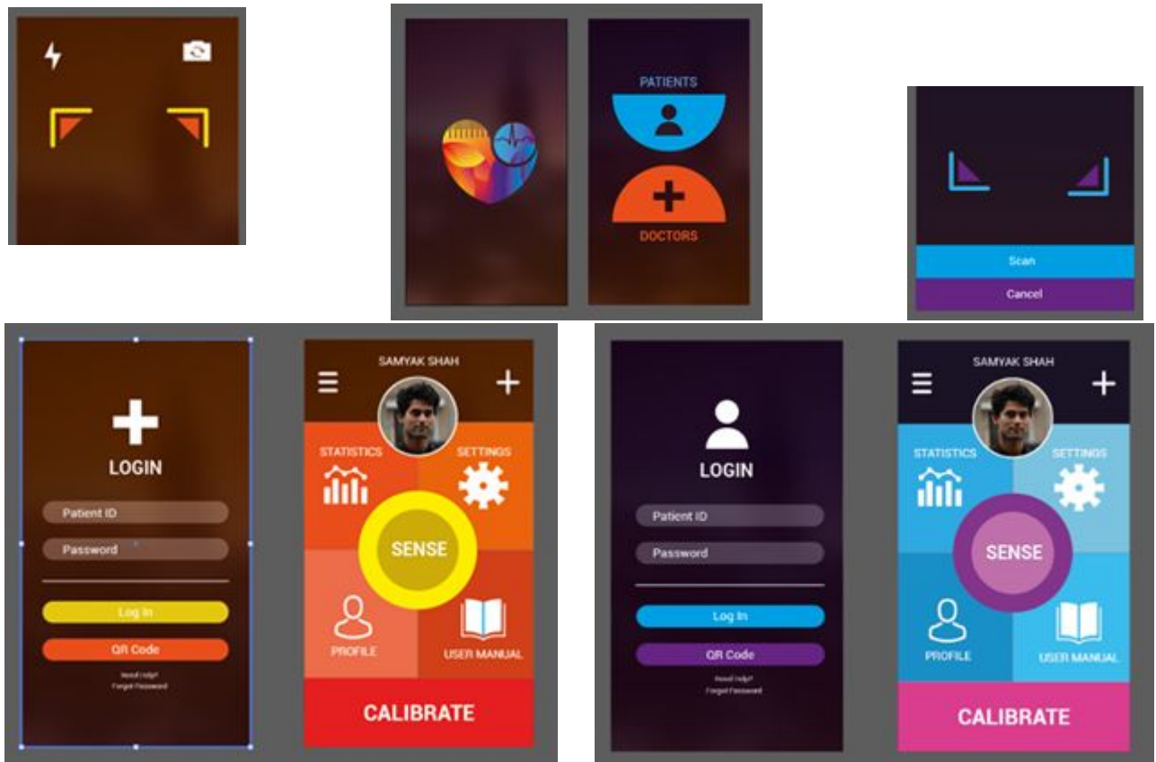
Figure 5: Template of app developed for Android smartphones, showing sections for doctors and patients, calibration, and statistics (e.g. weight and fluid balance recording by patient). Results can be sent to patient account, allowing specialists to view in real time, regardless of location.
