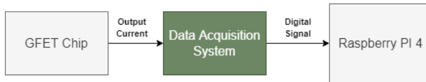
Figure 3. Simplified diagram of the measurement of the GFET's current by a custom-designed reading instrument with a further display of the results on Raspberry Pi 4.
