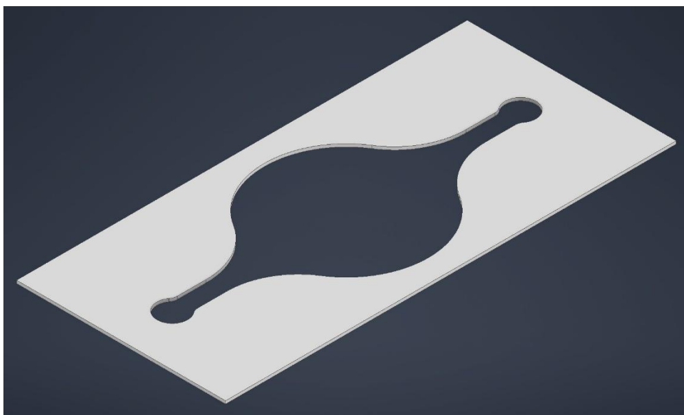
Figure S2. Three-dimensional (3D) model of the microfluidic channel.
