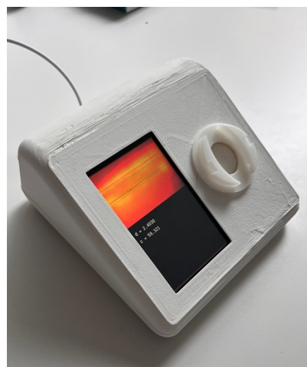
Figure 4: Reader device with integrated SPR setup and LCD screen showing CMOS output and correlated creatinine concentration.
