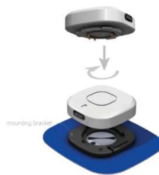
Figure 4: Palmsens' Sensit Wearable, an example of a modular potentiostat that can be attached and removed to a disposable microneedle patch (Palmsens)
