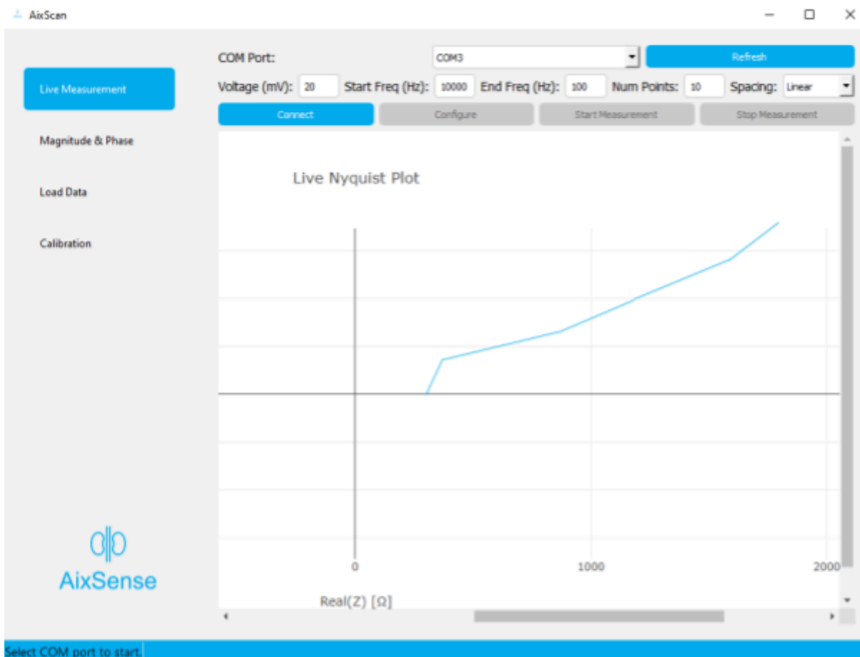
Fig. 8: Developed Graphical User Interface showing the Nyquist plot.
