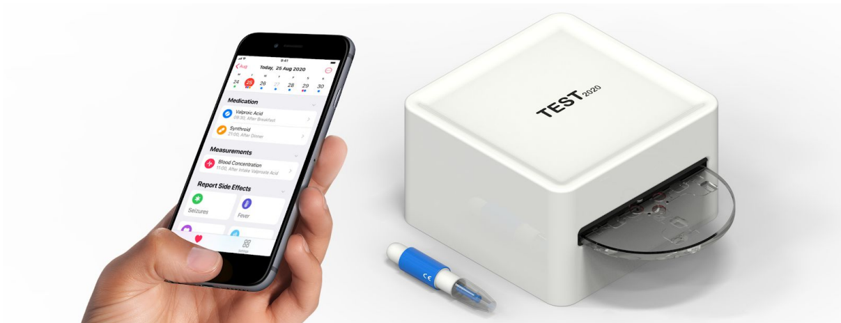
Fig. 1.3. On the left, the mobile application; on the right, the biosensor included with the cartridge and lancing device
