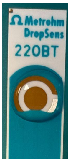
Figure 10. Beyond sufficient electrode coverage is achieved by application of a 100uL sample.
