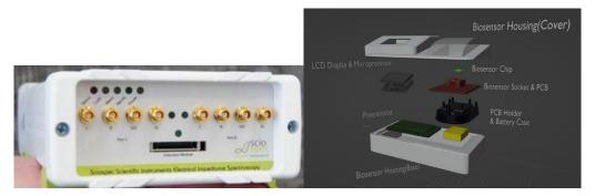
[Fig 5: Image our potentiostat device (Left) and 3D-render of the completed device (Right)]
