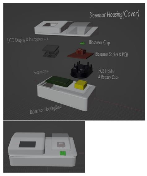
The figures show the **AixSense Reader's** design, which prioritizes the safeguarding of its core components. The sensitive biosensor chip is shielded from external contaminants, ensuring consistent and reliable readings. This structural integrity plays a pivotal role in maintaining the device's performance and longevity. The reader is sized approximately 20 cm x 30 cm x 30 cm.
