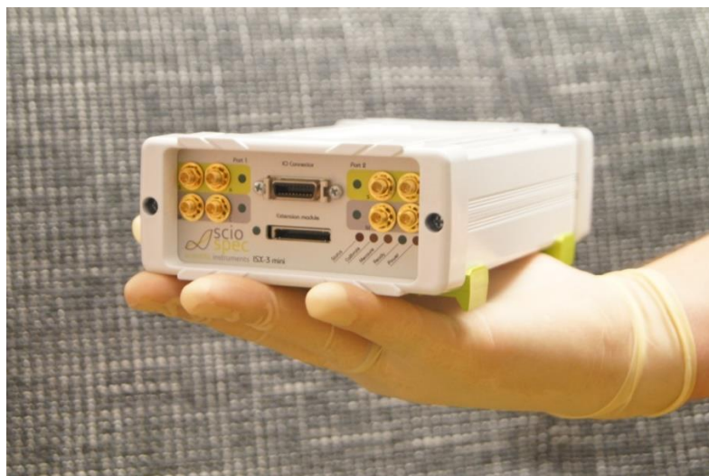
Fig.9 Electrical Impedance Analyzer for EIS measurements (Courtesy: Sciospec Scientific Instruments GmbH)
