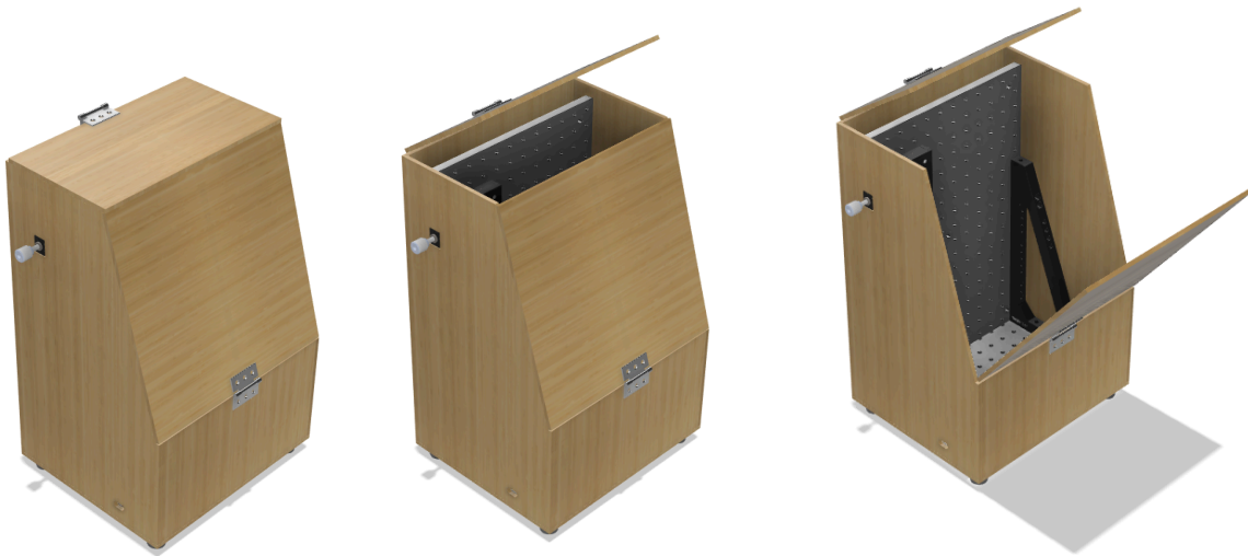
Figure 19: Model of the sensor case closed, with the top lid opened, and with the front and top lid opened
