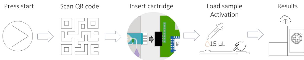
**Figure 3: Graphical representation of the workflow from start until results.**
