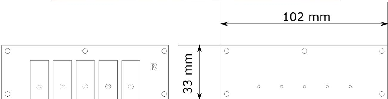
**Figure 10: picture and design of the incubation cell.** The cell is used for the incubation of functionalised AuNP. The cell is made from PMMA. Around the WE, there is a sticker made of PSA that sticks to the electrode and the PMMA to prevent leaking. At the end, the screws are tightened to assure a leak free incubation chamber.
