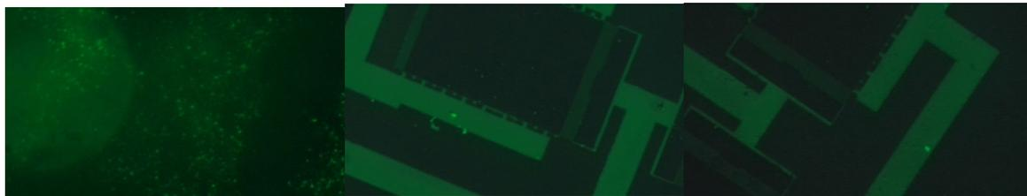
**Fig.9** FITC image of silanized ITO (left). Fluorescent measurement images of anti-GFAP immobilized sample (middle) and anti-GFAP – GFAP immobilized sample(right), x5 Magnification.
