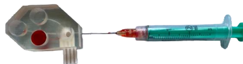
Figure 8: Microfluidic test with syringe.
