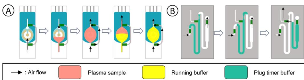
**Figure 5: Working principle of A) the air-bridge-mediated SPE incubation chamber, and B) the plug timer.**
