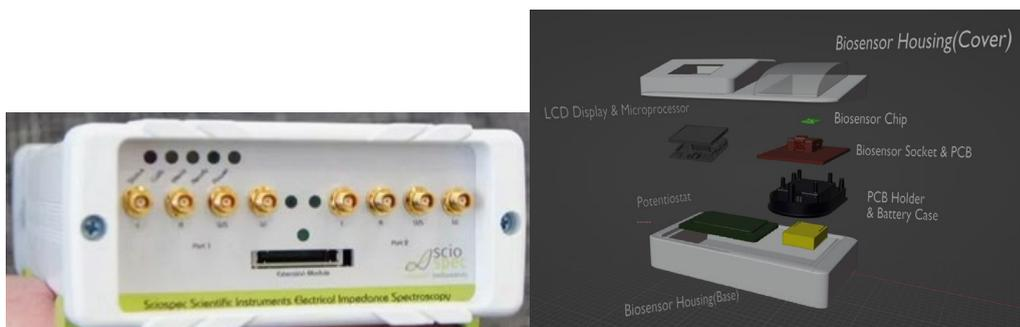
[Fig 5: Image our potentiostat device (Left) and 3D-render of the completed device (Right)]
