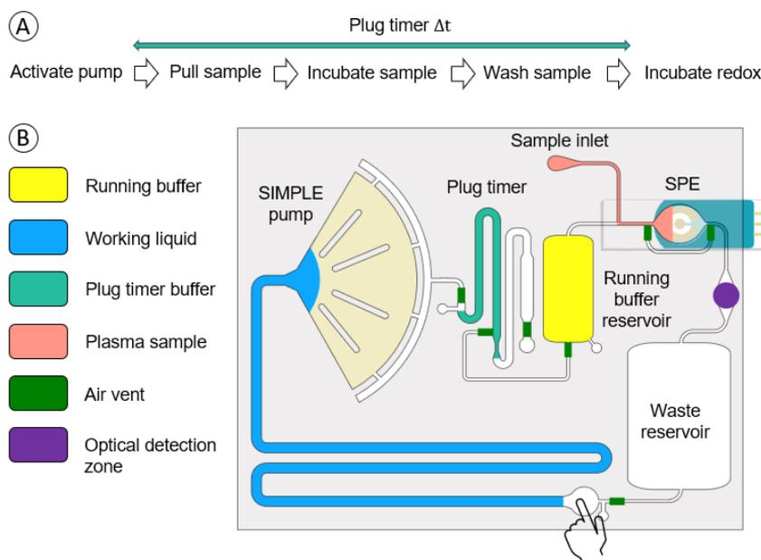
**Figure 2: Graphical representation of (A) the workflow and (B) the parts of the SIMPLE cartridge.**
