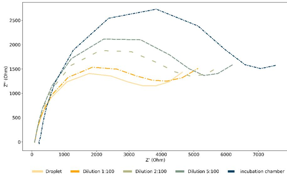
Figure 13: EIS graph showing difference in EIS signal between different colour dye dilutions and between droplet and incubation chambers.
