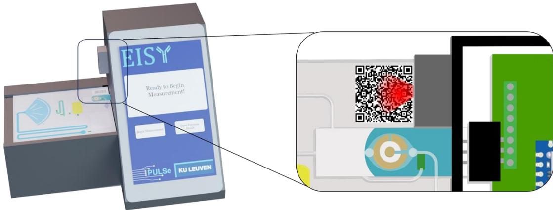
**Figure 14:** Graphical representation of the 2D barcode scanner, mounted on the side of the reader device above the cartridge. This is used to transfer chip specific calibration data to the device, which is needed to calculate the  $\Delta R_{CT}$  accurately.
