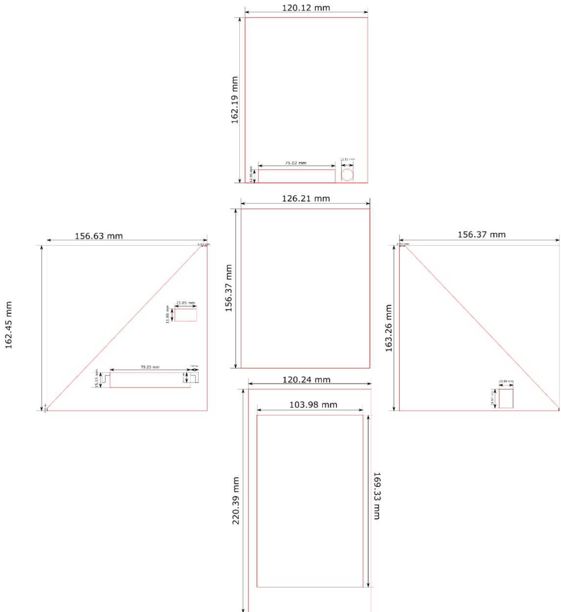
Figure 15: Dimensions of the reader device.
