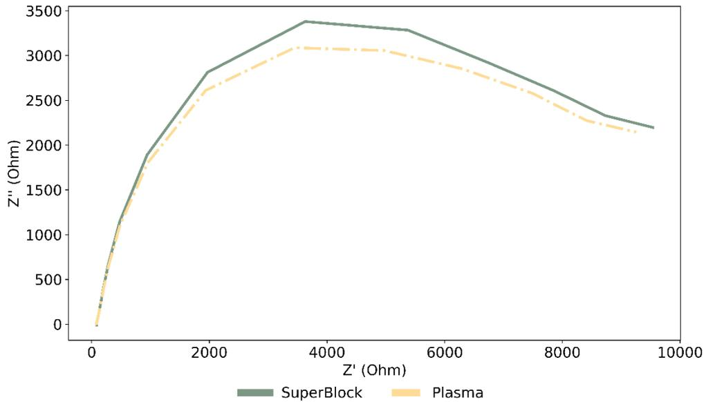
Figure 11: EIS graph showing resistance difference after plasma incubation. The fitted  $R_{CT}$  values have a difference of around 239 Ohms.
