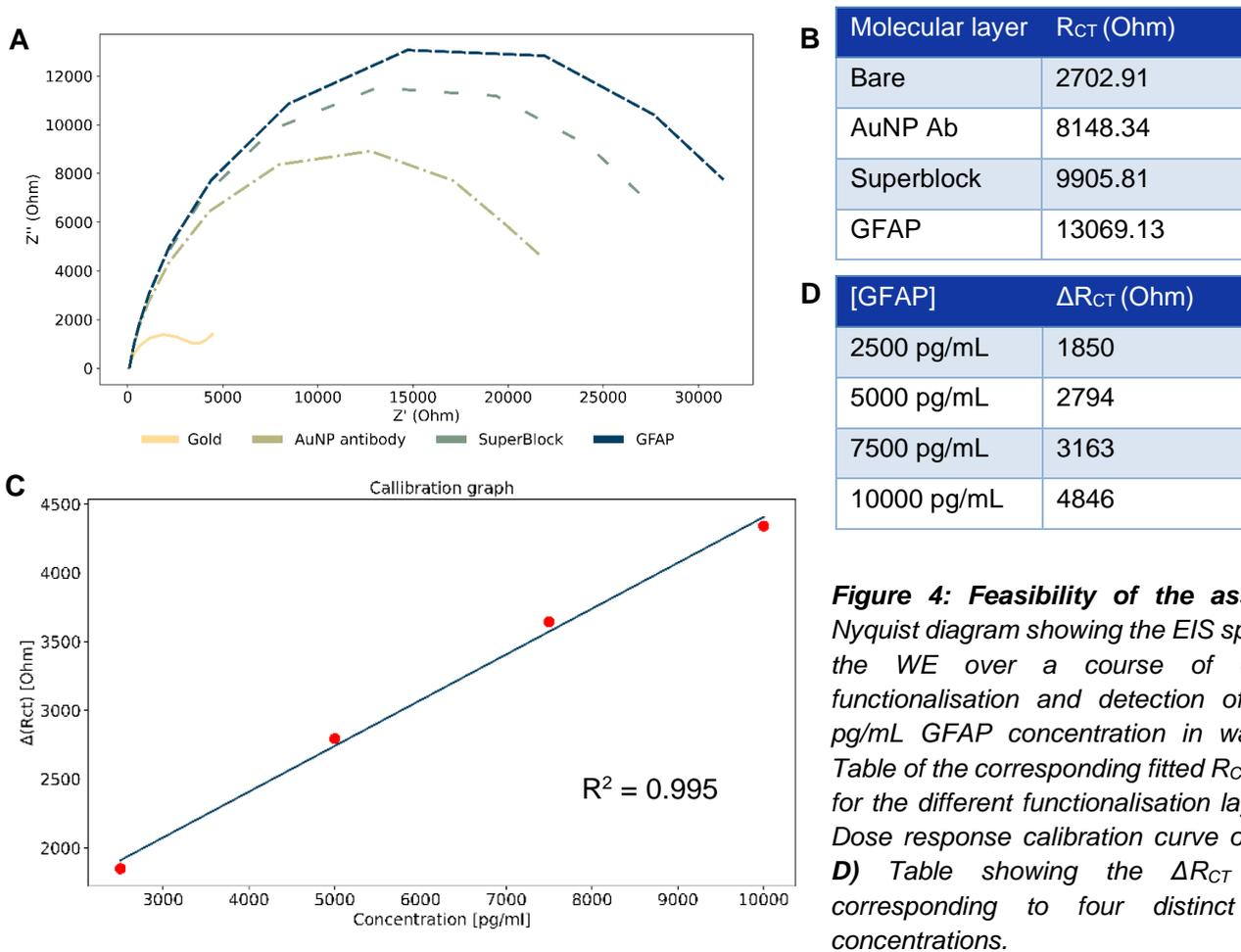
**Figure 4: Feasibility of the assay. A)** Nyquist diagram showing the EIS spectra of the WE over a course of different functionalisation and detection of 10000 pg/mL GFAP concentration in water. **B)** Table of the corresponding fitted  $R_{CT}$  values for the different functionalisation layers. **C)** Dose response calibration curve of GFAP **D)** Table showing the  $\Delta R_{CT}$  values corresponding to four distinct GFAP concentrations.
